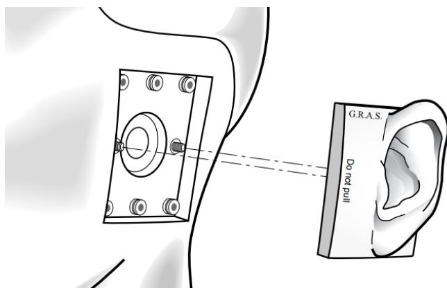
GRAS anthropometric pinna mounted on the 43AG test fixture's cheek plate using the RA0517 kit and finger screws (both included with the anthropometric pinna):
