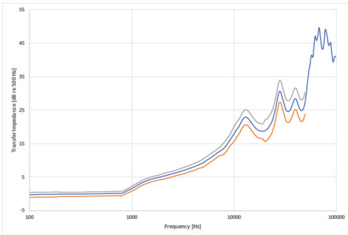
*Fig 1. The transfer impedance of a typical RA0404 Hi-Res Ear Simulator with tolerances. Up to 10 kHz, the response is within the limits defined by IEC 60318-4. Above 10 kHz, the response is within a fairly tight tolerance band up to 50 kHz*
