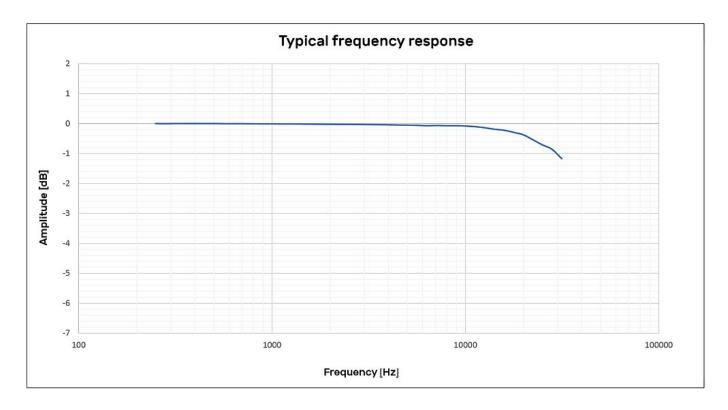
The frequency response is within ±3 dB up to 31.5 kHz
