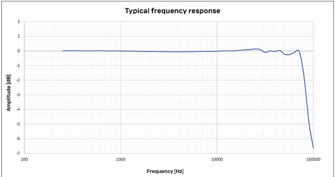
The frequency response is within  $\pm 3$  dB up to 70 kHz
