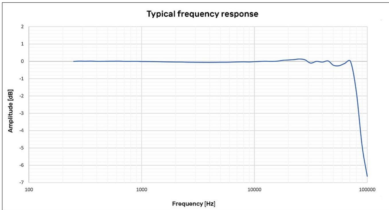
The frequency response is within  $\pm 3$  dB up to 70 kHz
