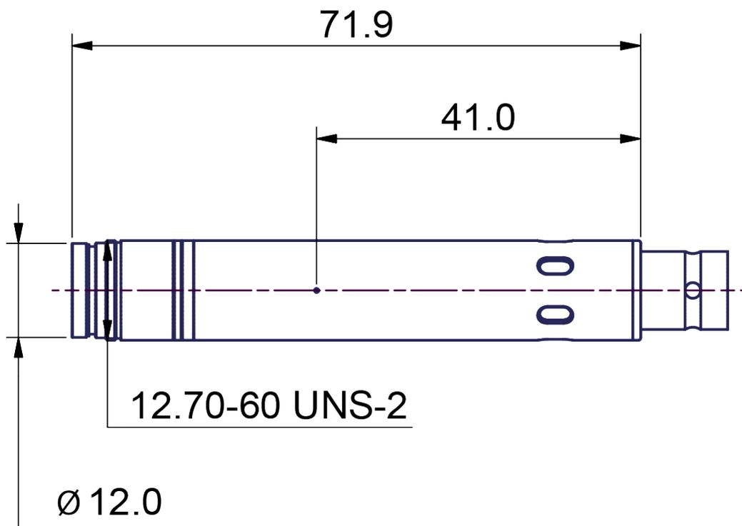
GRAS 246AE 1/2" CCP Free-field Standard SysCheck2 Microphone Set. This is the "standard" rear-vented version.
