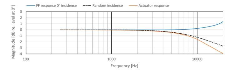
Typical frequency response (with protection grid)
