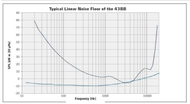
The noise floor (solid line) is typically below the threshold of human hearing (dashed line).
