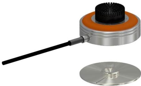
When the 147AX microphone set is placed over the mounting disc, a center guide ensures that the microphone will be attached and centered to the disc correctly once the magnetic force kicks in. In this way, it is easy to mount in difficult-to-access locations with no loss of placement accuracy.
