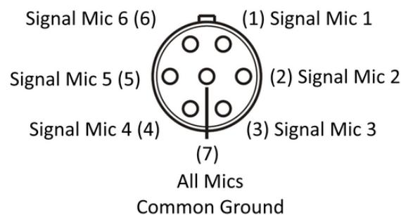
Array's structure 7-pin LEMO plug 1B female (external view)
