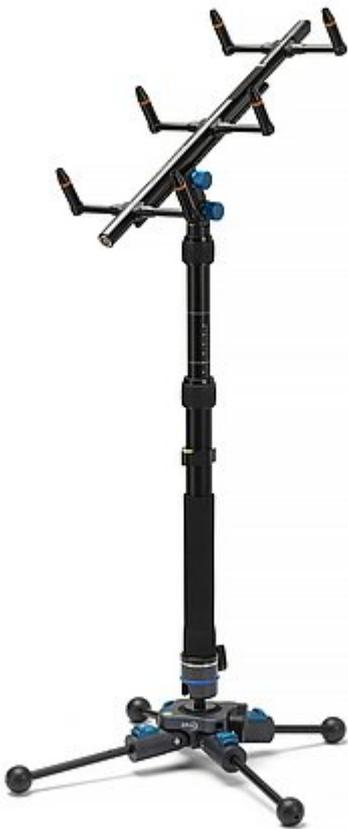
The GRAS PR0004 AutoArray is a rugged, six-microphone array purpose-built for accurate and repeatable in-cabin acoustic measurements. It features an "AES" configuration, aligned with the AES TC-AA (Audio Engineering Society Technical Committee on Automotive Audio) guidelines. This array enables high-resolution spatial analysis of vehicle interiors, giving automotive OEMs and audio engineers the tools to quantify and enhance cabin soundscapes.
