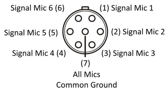
Array's structure 7-pin LEMO plug 1B female (external view)
