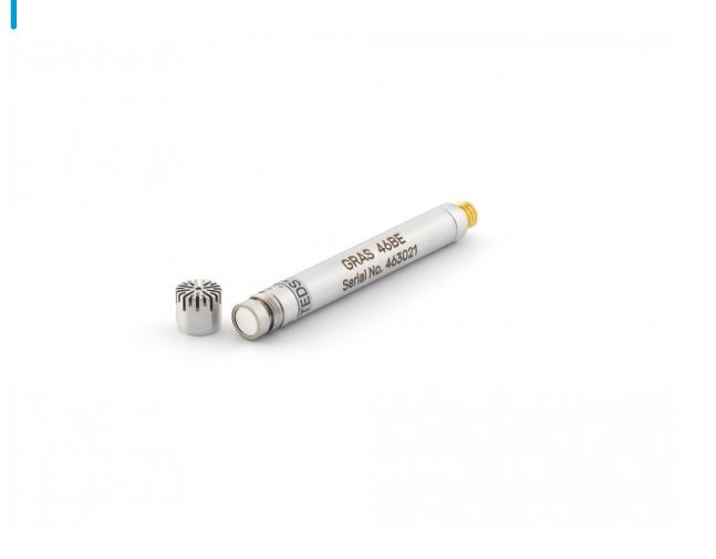
Freq range: 4 Hz to 80 kHz Dyn range: 35 dB(A) to 160 dB Sensitivity: 3.6 mV/Pa Use: For general acoustic diagnostics The GRAS 46BE is a ¼" Constant Current Power CCP freefield microphone set for measuring high sound pressure levels at high frequencies. It is terminated with a 10/32 UNC microdot female connector and is TEDS compatible. The equivalent traditional 200 V LEMO type is <u>GRAS 46BF</u> **NOTE:** Optimized for use without protection grid—remove grid before measuring.
