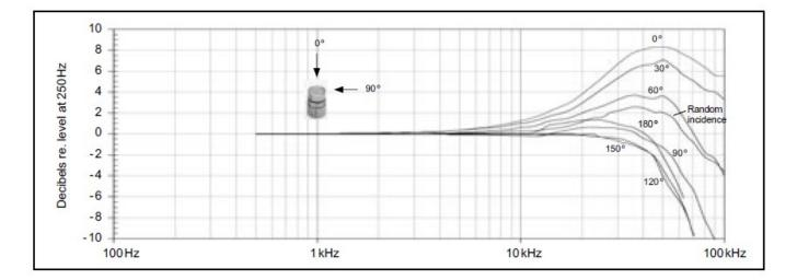
Free-field corrections for different angles of incidence
