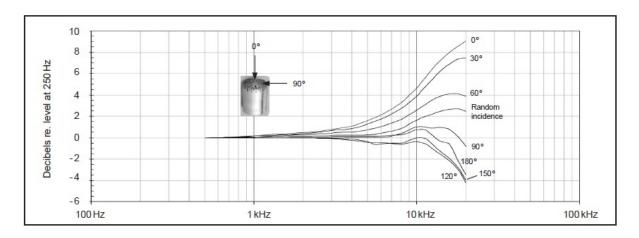
Free-field corrections for different angles of incidence
