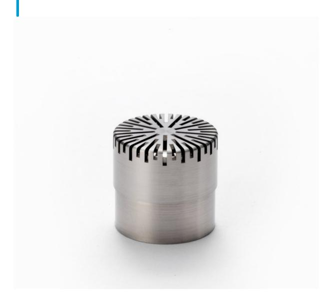
Freq range: 3.15 Hz to 40 kHz Dyn range: 20 dBA to 164 dB Sensitivity: 12.5 mV/Pa The 40AC is an IEC 61094 WS2F classified ½" externally polarized free-field, wide-frequency microphone with rearventing. The prepolarized equivalent is GRAS 40AM.
