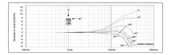
Free-field corrections for various degrees of incidence
