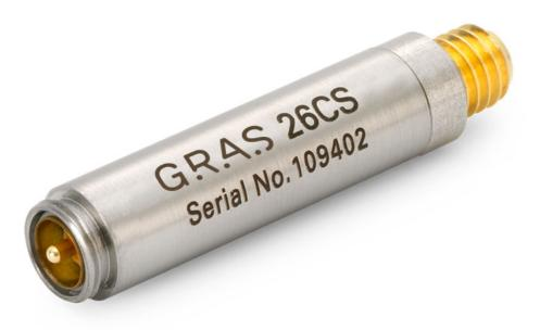
Freq range: 2.5 Hz - 200 kHz Noise: 1.8 µV Gain: -0.45 dB Special feature: For confined spaces The GRAS 26CS 1/4" Preamplifier is a very small preamplifier optimized for use with prepolarized condenser microphones. It is a robust unit and uses a CCP power supply. It has a very low inherent noise level, a large dynamic range and a frequency response from below 2 Hz to above 200 kHz.
