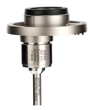
Connection: 0 V/CCP Volume: Complex Dyn range: 25 dB(A) to 150 dB ANSI: S3.7 The GRAS 43AE-S1 Ear Simulator according to ITU-T Rec. P57 Type 3.2, Prepolarized is for acoustically testing supra-aural earphones, telephone handsets and loudspeakers, and complies with the international requirements: ITU-T Recommendation P.57 (08/96) "Serie P: Telephone Transmission quality. Objective measuring apparatus: Artificial ears".
