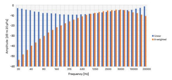
Typical noise floor shown in 1/3-octave bands - linear and A-weighted
