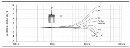
Free-field corrections for different angles of incidence
