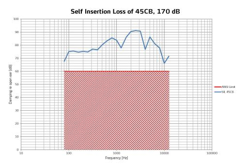
Self Insertion Loss, Measured with closed ear simulators: 100 Hz – 8 kHz >74 dB Self Insertion Loss, Measured with closed ear simulators: 80 Hz – 12.5 kHz >65 dB
