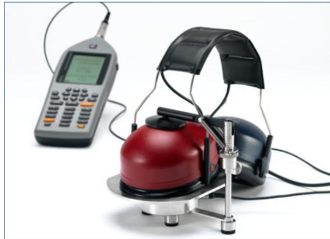
*HDA-200 Circum-aural earphones mounted on the IEC 60318-2 Ear Simulator (high-frequency coupler). This setup is based on a 1/2" measurement microphone.*
