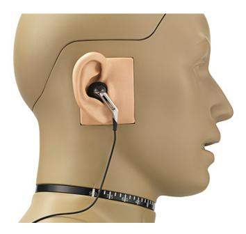
Connection: Traditional Power Supply (200 V/LEMO) Channel(s): 2 ANSI: S3.36 Based on IEC 60318-7 Based on ITU-T Rec. P.58 The 45BB-12 KEMAR is an acoustic research tool with a built-in low-noise ear simulator for testing of ear and headphones and in-ear ear protectors with or without active noise cancellation. Its corresponding single-channel equivalent is <u>GRAS 45BB-11 KEMAR with Anthropometric</u> <u>Pinnae for Ear- and Headphone Test, 1-Ch LEMO.</u>
