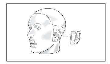
Standard pinnae are push mounted from the outside. The anthropometric pinnae, however, are secured from the inside by two screws in addition to the push mounting.
